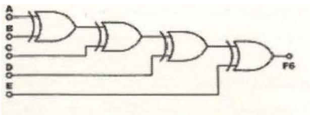
Fig. 9-2-3 Even parity generator circuit
