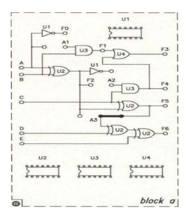
Fig. 9-2-2 Wiring diagram (KL-26002 block a)
