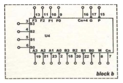
Fig. 9-1-3 Wring diagram (KL-26005 block b, U4=74181)
