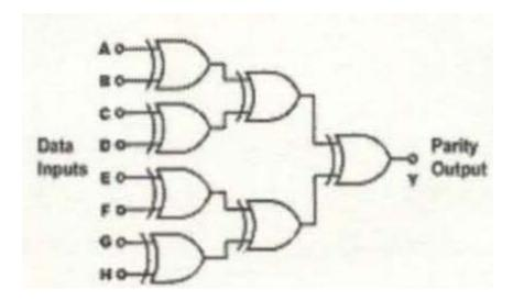
Fig. 9-2-1 Even parity generator circuit
