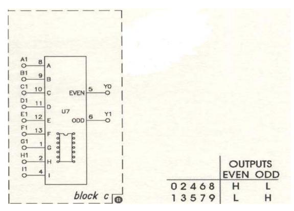
Fig. 9-2-4 Wiring diagram (KL-26005 block c)
